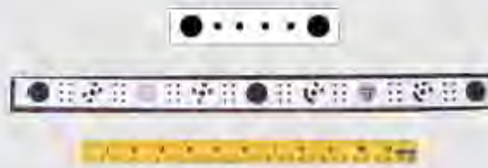
Figure D.7. Examples of calibrated target sticks (CTS) and an object of known length. The center CTS contains circular bar codes, which are used by some three-dimensional measuring and mapping software and assist with the initial image orientation process.
